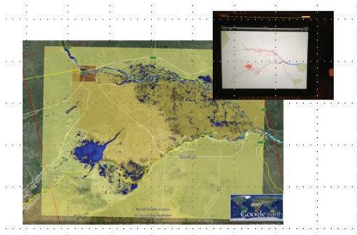
**Fig. 6: Radarsat automated tiled water extent display along with corresponding Ipad display**
