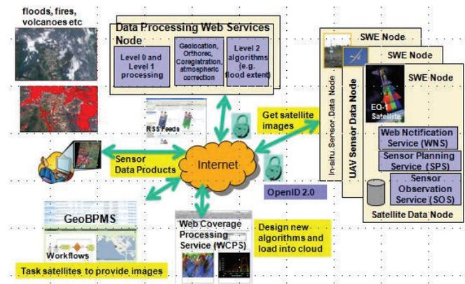
Fig. 2: SensorWeb high level architecture
