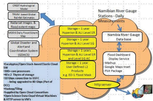
Fig. 3: Cloud computing service being used for Flood Pilot and some of the functionality that the team integrated
