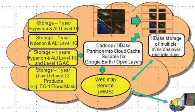
Fig. 4: Key function on the cloud is the use of Hadoop for tiling of large data sets
