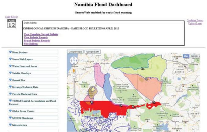
Fig. 5: Namibia Flood Dashboard with MODIS data layer, water lines and water catchments layer enabled
